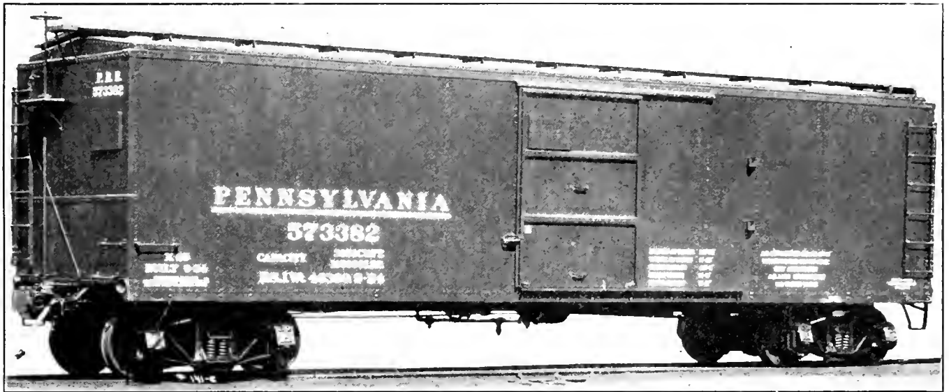
All Steel Double Sheathed Box Car Built for the Pennsylvania Railroad Co. by the Bethlehem Steel Co.
